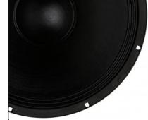
800 W continuous program power capacity 76 mm (3 in) copper voice coil 40 - 3000 Hz response 98.5 dB sensitivity Ventilated voice coil gap for reduced power compression
