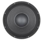
This next evolution subwoofer uses a new, longer, four layer aluminum voice coil. The result is less heat, more energy in the gap, higher sensitivity, higher power handling, lower distortion and better overall performance. The 15DS100 features a 37mm long, 4 inch diameter (100mm) Copper Clad Aluminum Wire voice coil. With a 1500watt AES power rating, 96.8 dB sensitivity, and over 14.0mm of Xvar, this high energy subwoofer is a significant step forward from similar models in the B&C range.
