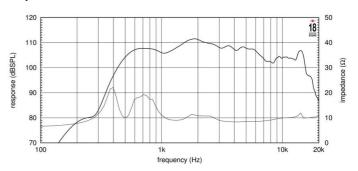
FREQUENCY RESPONSE MEASURED WITH 2.83 V INPUT ON AXIS AT 1 METER DISTANCE FROM THROAT OF XR2064 HORN. IMPEDENCE MEASURED ON SAME HORN.
