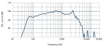
Frequency response curve of the loudspeaker make in a hemispherical, free field and mounted in a reflex box with an internal volume of 50 litres and tuned at 60Hz, applying a sinusoidal signal of 2.83 V @8 at 1m.
