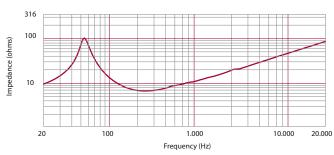
Impedence magnitude curve measured in free air
