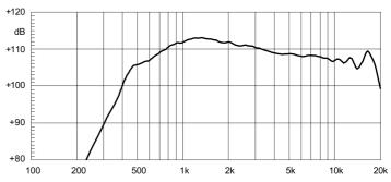
ND1460A MEASURED WITH 1W INPUT ON RATED IMPEDANCE AT 1 M DISTANCE ON AXIS FROM THE MOUTH OF XT1464 HORN
