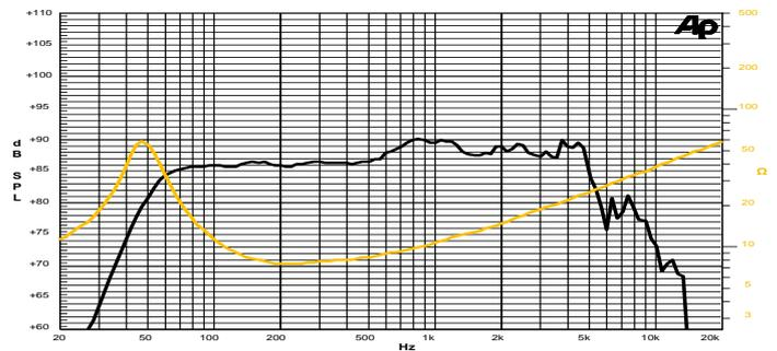
Frequency Response on 18 Lt @ 50 Hz Vented Box @ 1W, 1m
