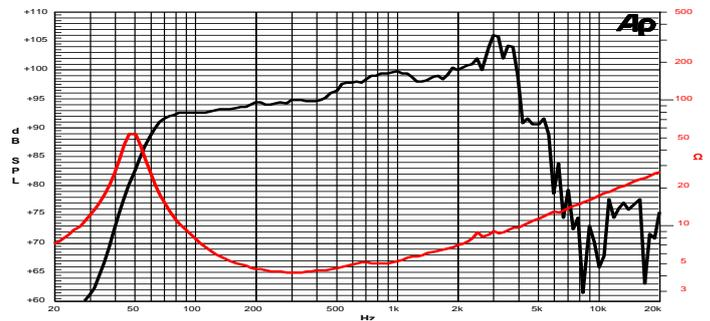
Frequency Response on 35 Lt @ 60 Hz Vented Box @ 1W, 1m
