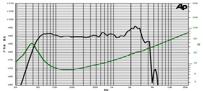
Frequency Response on 60 Lt @ 45 Hz Vented Box @ 1W, 1m
