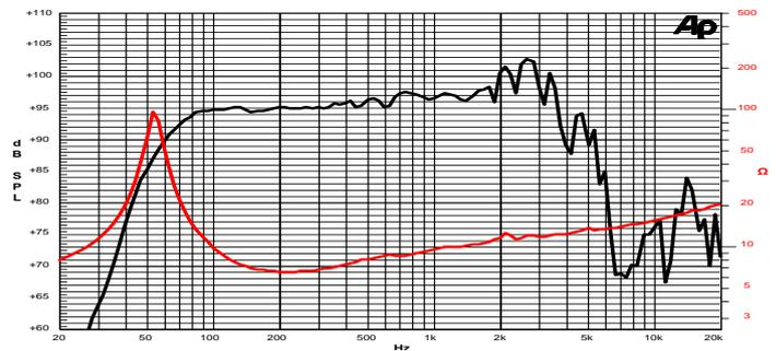
Frequency Response on 45 Lt @ 55 Hz Vented Box @ 1W, 1m
